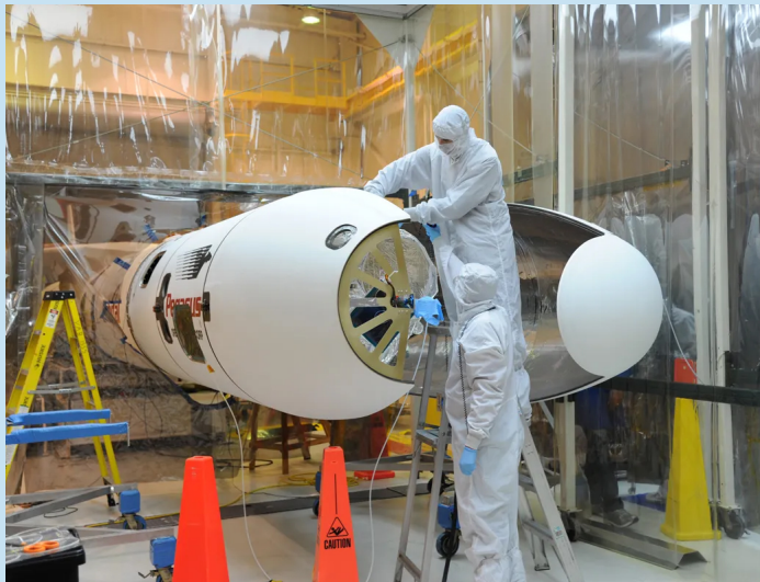
The fairing is installed on the NuSTAR satellite to protect it as it travels through the atmosphere and into space. Image credit: U.S. Air Force/Doug Gruben
