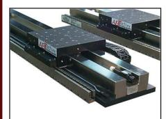
Air bearing linear slide for lithography machine application. Magnetically preloaded for low profile with linear motor drive and optical encoder.
