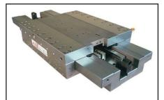
Fully captured apposing pad Air Bearing linear slide for high stiffness and accuracy. Constructed of hardened 440C stainless steel with linear motor drive and optical encoder.
