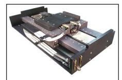
Fully captured apposing pad air bearing linear slide design for high stiffness and accuracy. Constructed of hardcoated aluminum with linear motor drive and optical encoder.
