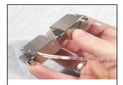
Miniature linear air bearing slide with magnetically preloaded carriage. Smooth motion in a small package.
