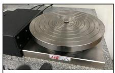
Grind table: ABTech's motorized wet grind tables are ideal for use in light grinding applications giving our customers the flexibility to turn their conventional surface grinding machine into a radial face grinder.
