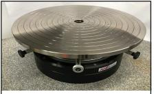
Portable rotary table: ABTech's AT-400 portable rotary air bearing table with 8 Knob 600mm tilt and center worktable is ideal for inspection of large diameter parts up to 32" diameter and 2,000 lbs.
